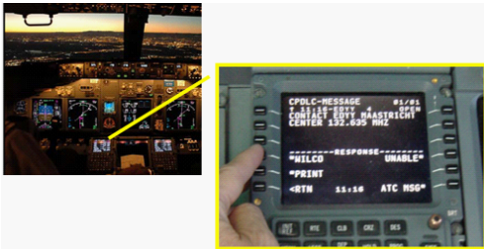
Figure 1. Controller-Pilot Data-Link Capability Demonstration.
