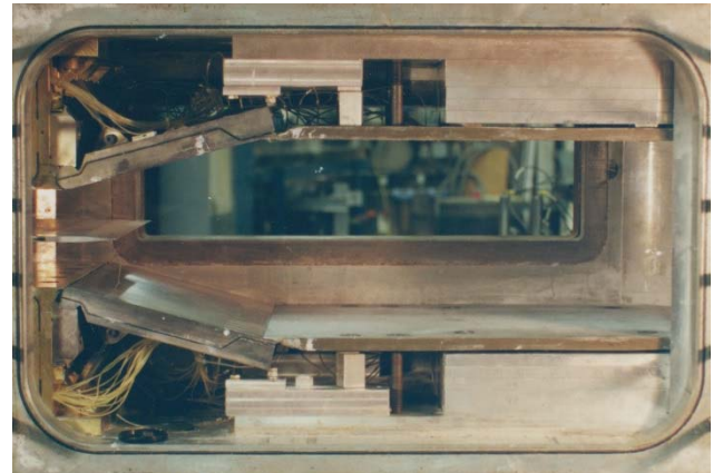
a) Upstream Splitter Plate portion of test section b) Downstream Wake region of test section Fig 4 Side view of test section (viewed from the East, flow left to right)
