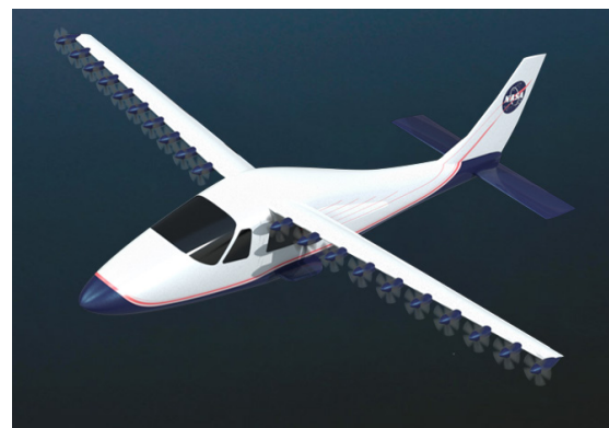
Figure 4 – Artist depiction of SCEPTOR-like aircraft with high-lift system active (47).
