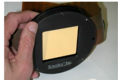
Figure 5: 64 x 64 element DM with a fused silica facesheet. Trauger et al. , Proc. SPIE 8151, 81510G (2011).
