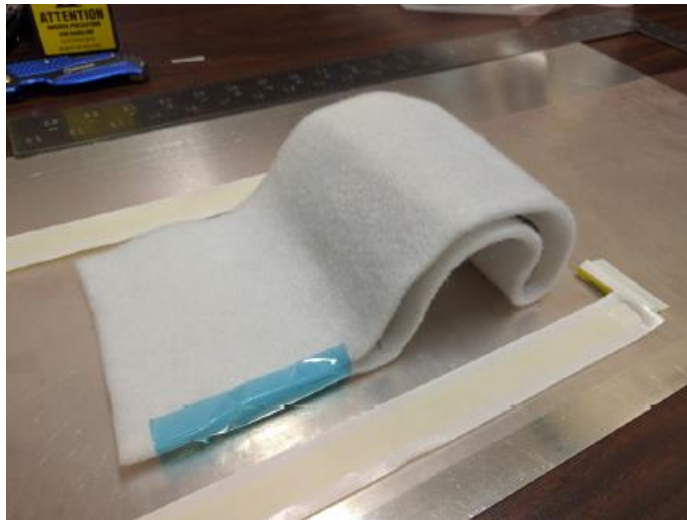
Composite panel surrounded by breather fabric
