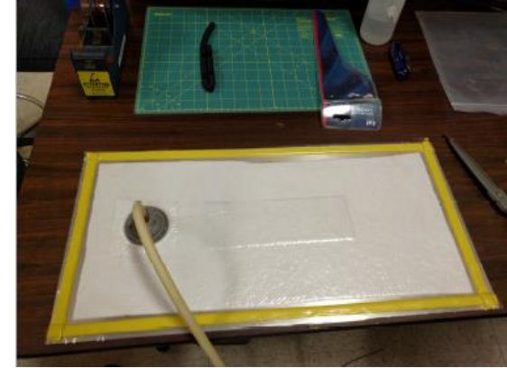
Flat panel fabrication: vacuum bagging
