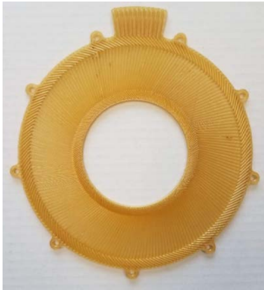
FDM from Extem (Tg of 311°C) (left) and Ultem 1010 (TG of 217°C) (right) FDM filament.
