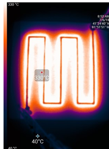
Direct Printed Silver Coils - High Current Test
