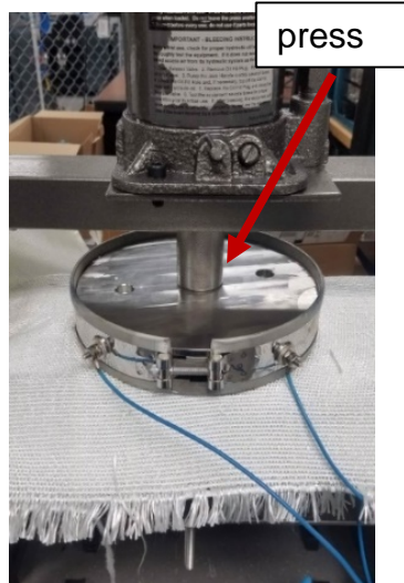
Pressing process needed to further densify the stator
