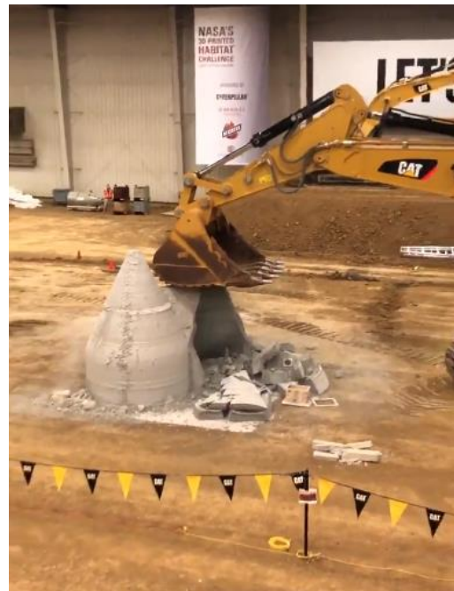
Figure 16. Onsite tests of printed habitats (top to bottom): smoke test, impact test, and crush test.
