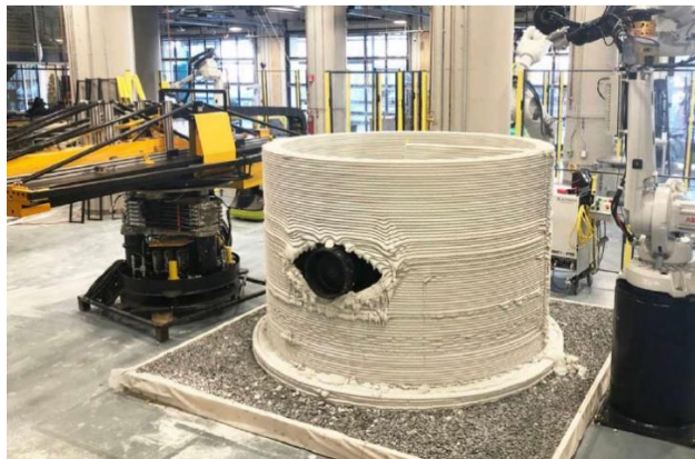
Figure 13. Habitat element printed by SEArch+/Apis Cor.
