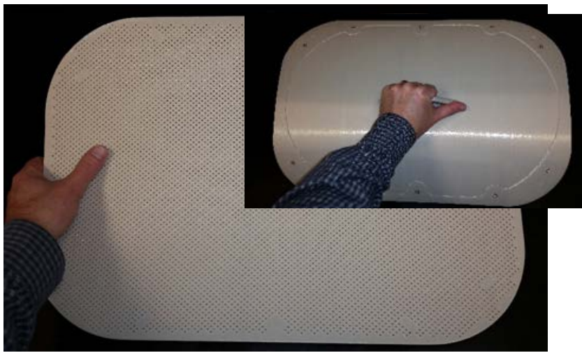
Engine Panel Access Door
