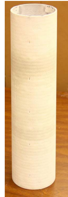
SiC/SiC Combustion Liners: Outer Liner and EBC Coated Inner Liner
