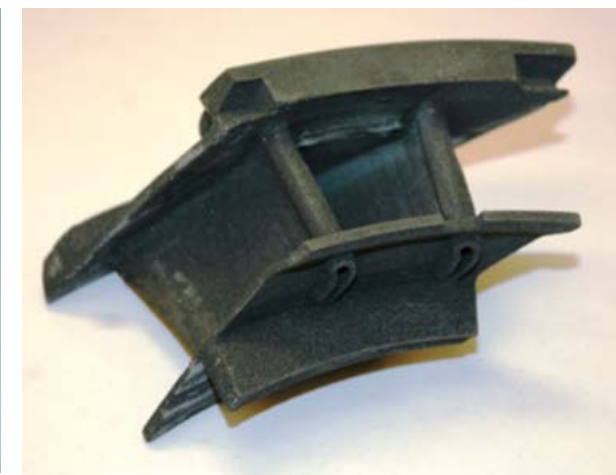
High pressure turbine cooled doublet vane sections.
