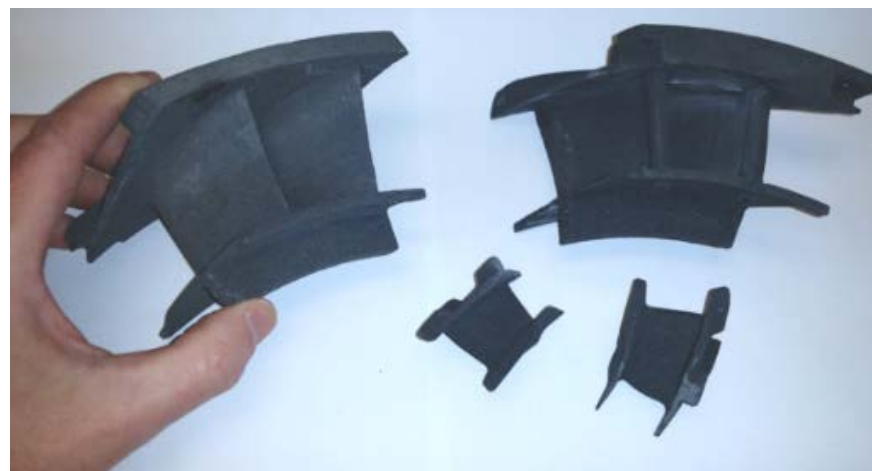
High pressure turbine cooled doublet vane sections.
