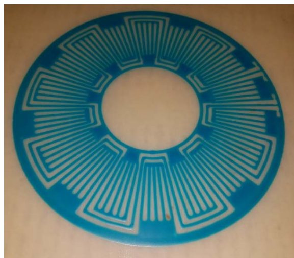
Direct Printed Dielectric Layer
