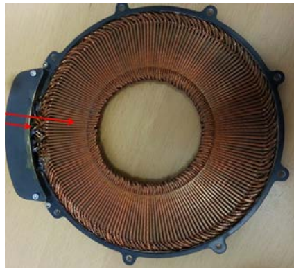
Litz Wire Coreless Stator
