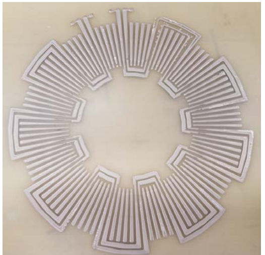
Direct Printed Silver Conductor Layer
