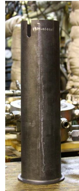
SiC/SiC Combustion Liners: Outer Liner and EBC Coated Inner Liner
