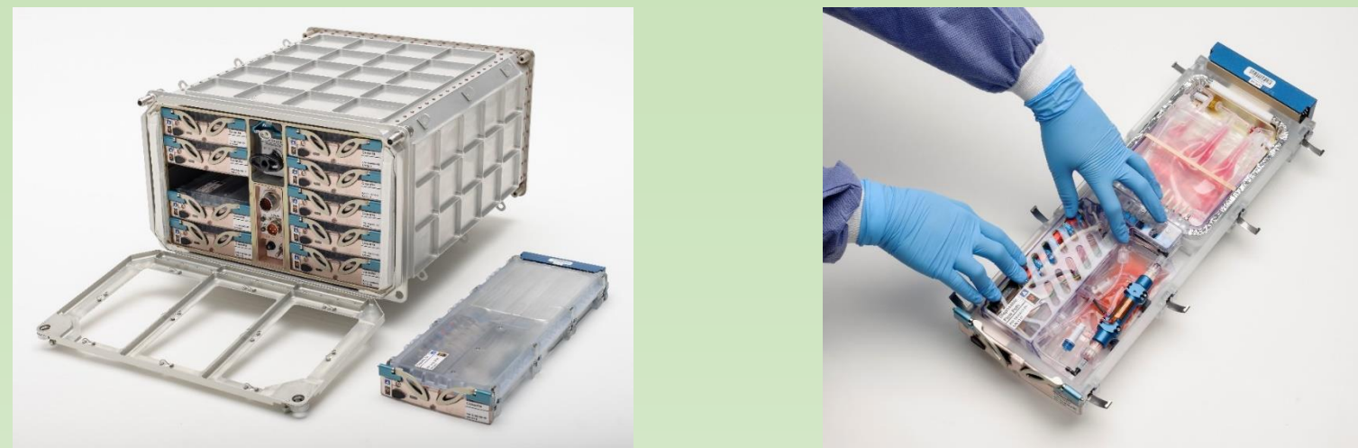
Figure 1. The current Bioculture system with a single bioreactor per cassette. Hart, Dominic. (2016). Bioculture System https://www.nasa.gov/sites/default/files/atoms/files/bioculture-fs_03oct2016.pdf
