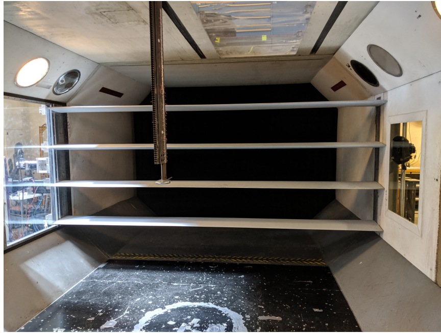
Figure 2. Gust Generator in Kirsten Wind Tunnel at University of Washington
