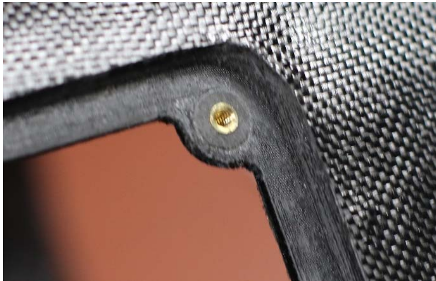
Figure 12. Brass Insert Embedded Into Nylon
