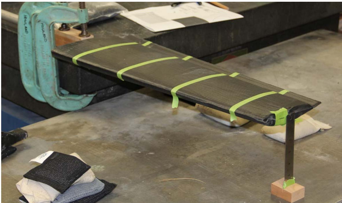
Figure 22. Foam Core Carbon Fiber Forward Wing Load Test Article
