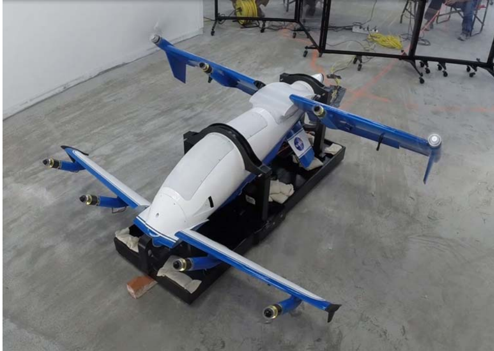
Figure 47. LA-8 Secured During Thermal Testing
