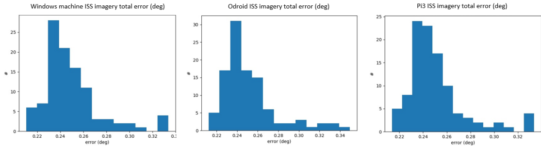
Figure 3: Total error histograms for the ISS data with the Windows machine on the left, Odroid in the middle, and Pi3 on the right
