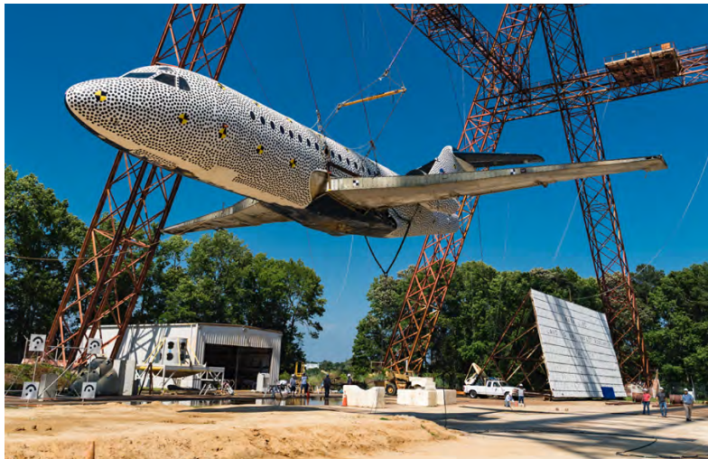
Figure 9. Photograph of the F28 as it is being lifted to the drop height. Note that the port side was painted white with 3-in.-diameter black dots added for photogrammetry.
