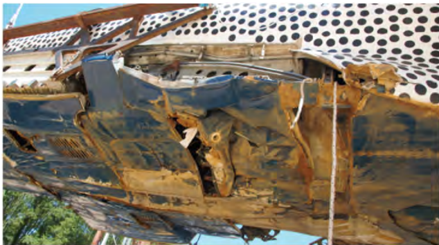
(a) Photograph of airframe damage.
