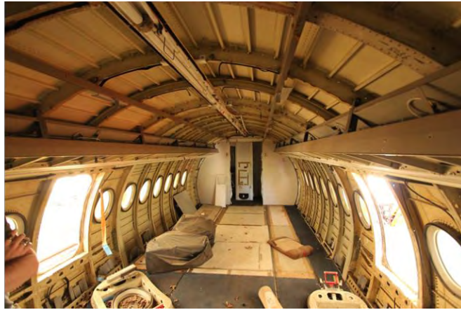
Figure 5. Interior view of the F28 aircraft, following removal of equipment by CanadaAir.
