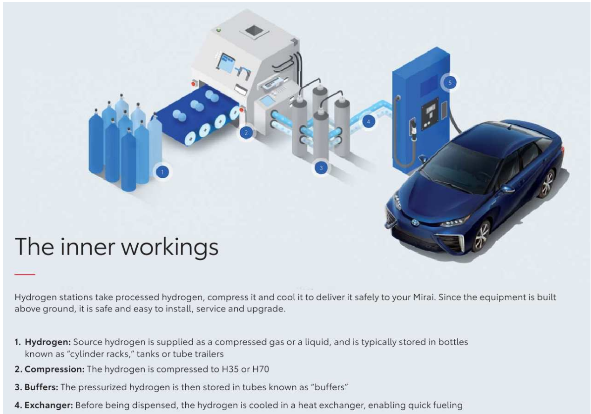
Figure 8: Toyota Mirai refueling diagram taken from the Yr-2018 sales brochure).
