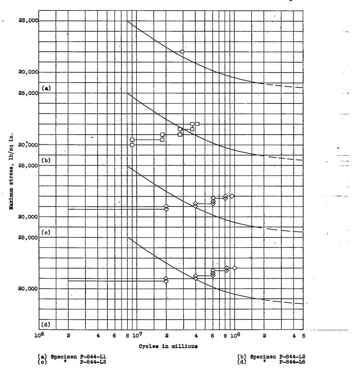
Figure 2.- Rotating-beam fatigue tests of 1.375-inch-diameter specimens of 178-T aluminum-alloy rod.
