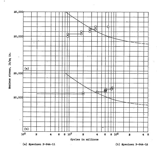
Figure 3.- Rotating-beam fatigue tests of 0.300-inoh-diameter specimens of 178-T aluminum-alloy rod.
