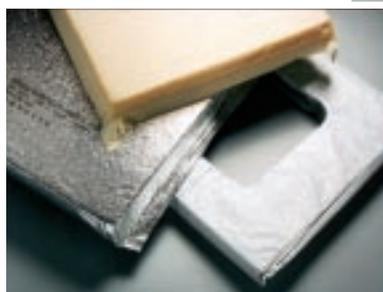
*Polyimide foam created for the Space Shuttle program can be fabricated for an assortment of industrial and commercial uses.*
