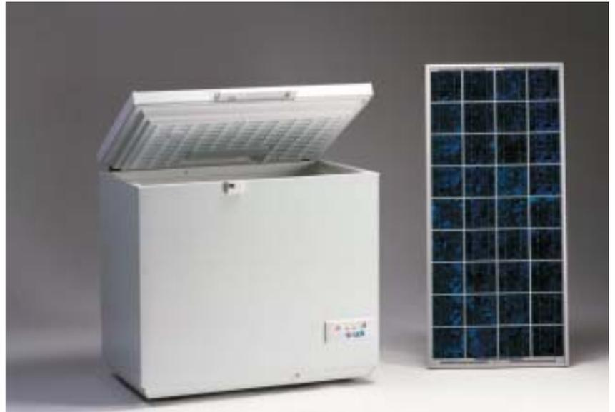
Designed to function in arid to semi-arid regions with at least 5 sun-hours per day, the photovoltaic, direct-drive SunDanzer™ solar refrigerator is a chest-type cabinet with a 105-liter internal volume, a lockable top-opening door, a corrosion-resistant coated steel exterior, and a patented low-frost system.
