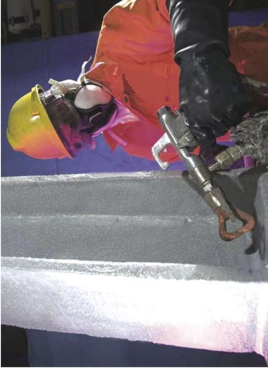
Fabrication shop application of Interchar fireproofing material to structural steel beams. Since Interchar is typically applied at a thickness between 1 and 8 millimeters, it does not impact the overall shape of the steel. This means architects and building planners can still explore intricate and innovate architectural designs.
