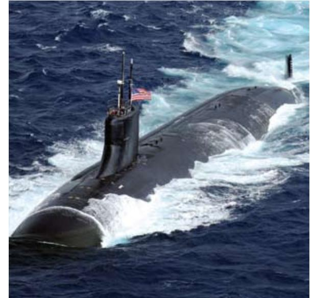
The U.S. Navy's Seawolf class submarines feature a “swim-by-wire” system adapted by NASA partner Draper Laboratory from the Lab's work during the DFBW program.
