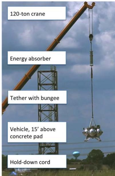
**Figure 3 – Morpheus 1.5B in Tether Test Configuration**
