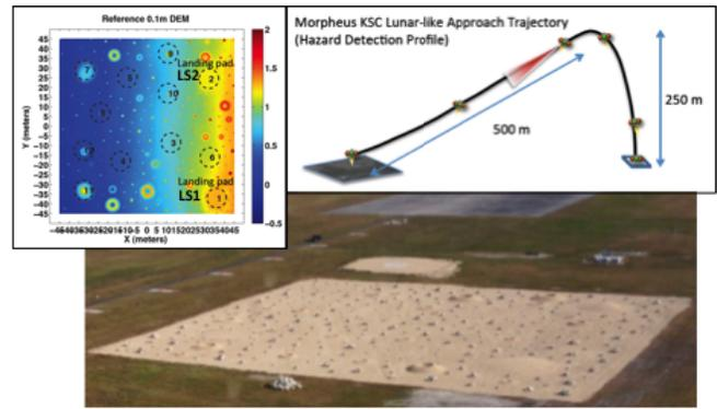
**Figure 7 – HDP Trajectory and Hazard Field Overview**
