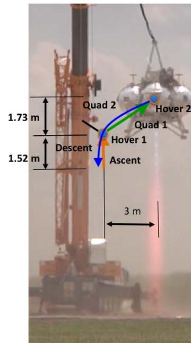
**Figure 10 – Tether Test 28 and 29 Profile**
