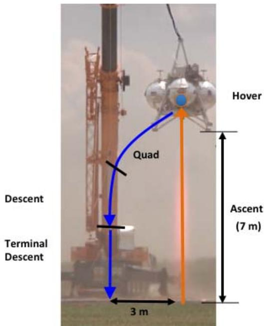
**Figure 5 – Ground Take-off And Landing (GTAL) Profile**
