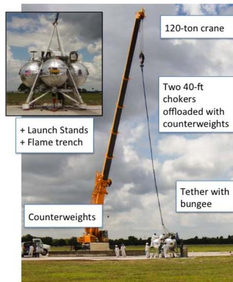
**Figure 4 – Ground Take-off And Landing (GTAL) Test Configuration**
