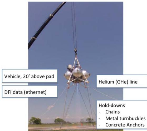
**Figure 1 – Morpheus 1.5B in Hot-Fire Test Configuration**
