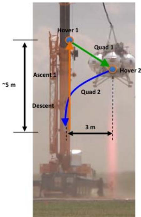
**Figure 11 –Tether Test 30, 31, and 32 Profile**
