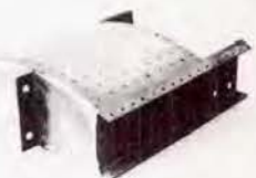
FIGURE 5. PROTECTIVELY COATED MOLYBDENUM ALLOY ASSEMBLY STRUCTURALLY TESTED AT 2500°F.
