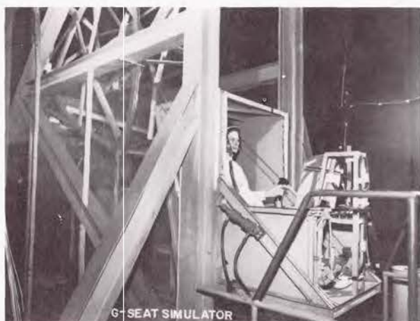
Figure 12. The North American Aviation (Columbus) "G-seat." (Courtesy of North American Aviation, Inc.).
