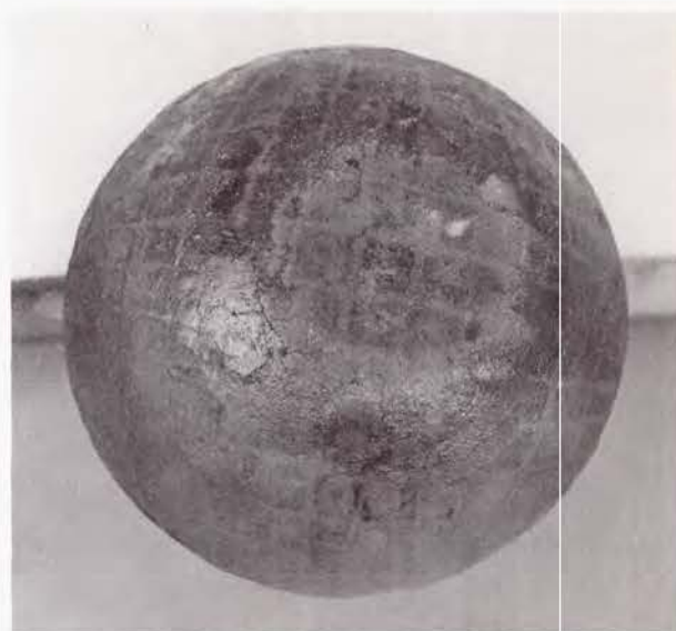
FIGURE 19. UNDERCUT SILICONIZED GRAPHITE TEST SPECIMEN COATED WITH ZIRCONIA AFTER TESTING AT 3800°F.
