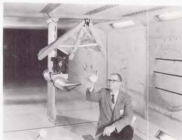
Figure 3.- Wind-tunnel setup for determination of line loads and complete glider static aerodynamic characteristics.
