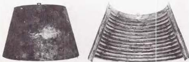
FIGURE 12. PROTECTIVELY COATED D-14 COLUMBIUM ALLOY COMPONENT AFTER EXPOSURE AT 1900° F.
