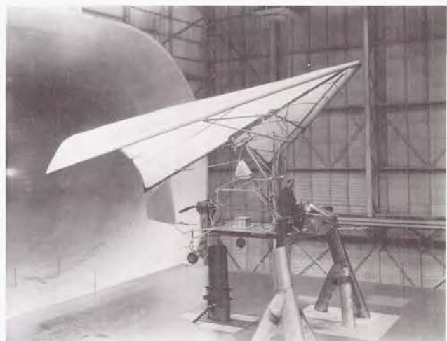
Figure 9. - Ryan flexible-wing vehicle setup for force tests in the Langley full-scale wind tunnel.
