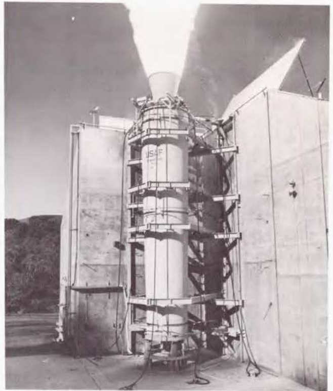
FIGURE 8. UTC TEST OF 2-SEGMENT MOTOR
