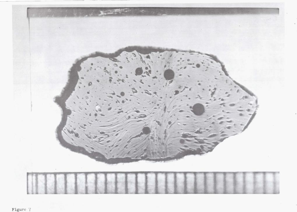
Shadowgram of a section cut through the center of an Ivory Coast tektite. The scale divisions are in millimeters.
