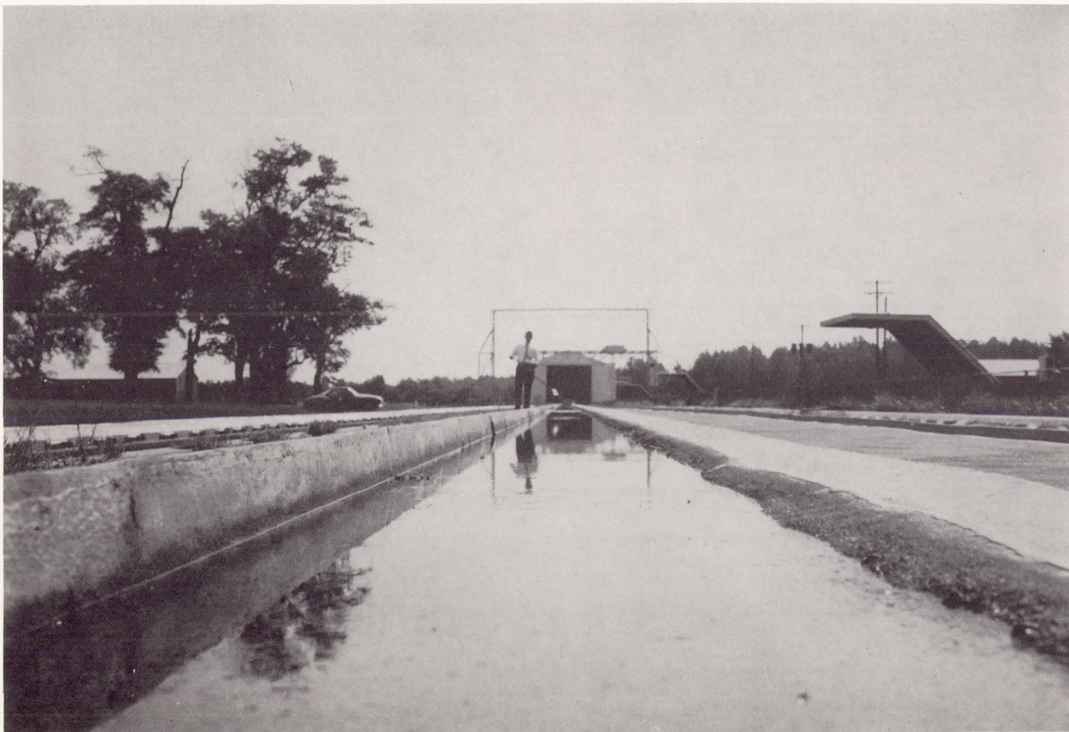
Figure 9.- Water-covered concrete runway immediately before wheel-braking run. d_1 = 0 to 0.3 inch.
