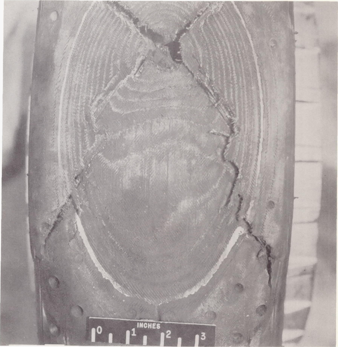
Figure 22.- Tire appearance after skidding approximately 60 feet on a dry concrete runway.
