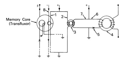
The problem: A highly reliable sense amplifier was desired for a computer magnetic core (transfluxor) used as a memory element. The output current from the memory was not sufficient to operate directly in the arithmetical section of the computer; it was therefore necessary to amplify the data from the memory before it could be used in the computer.
