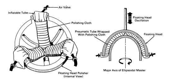
**The problem:** Quantity production of high-quality, thin-walled, ellipsoidal optical reflectors. For use in solar simulators, the inside surface of each reflector was required to be an ellipsoid of revolution about the major axis. Dimensions were: major axis, 20 inches; minor axis, 16 inches; and wall thickness, 1/4 inch.
