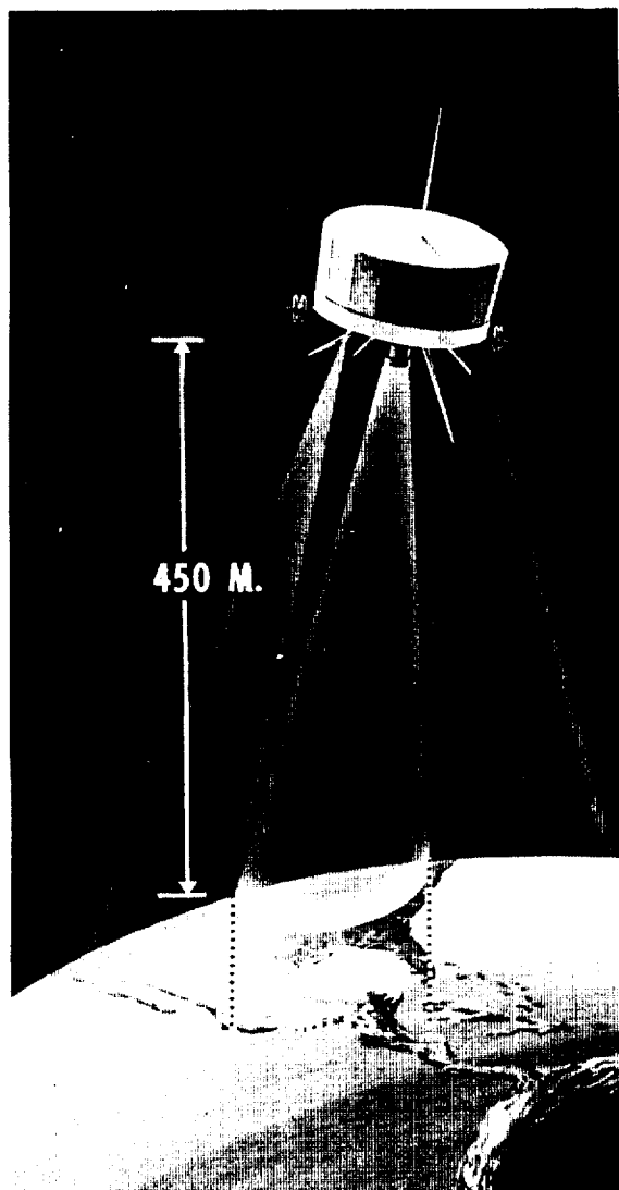
FIGURE 5-13. Tiros Sensors. Two TV cameras detect cloud cover; multichannel scanning radiometer detects water vapor, night clouds, reflected sunshine, and emitted heat, and permits low-resolution cloud mapping; nonscanning radiometers detect total radiation and thermal radiation.
