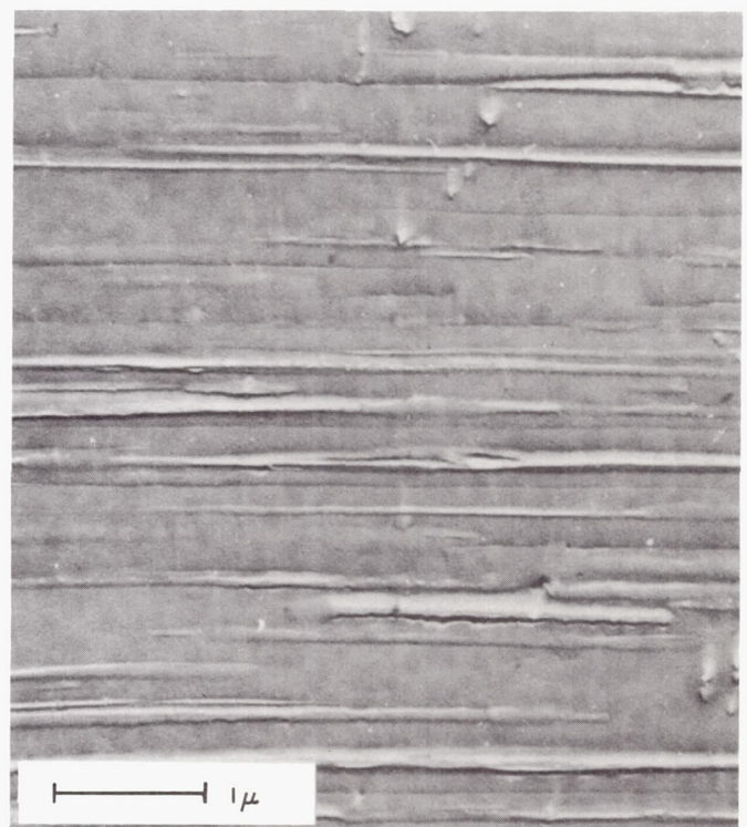
Fig. 5. Electron micrographs of edge of basal planes of pyrolytic graphite after various amounts of deformation at 2760°C lot 170
