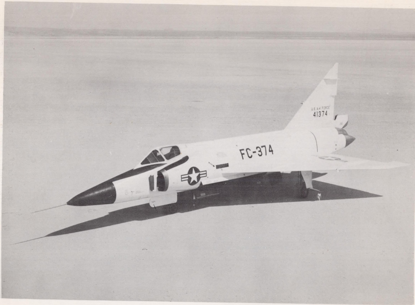
Figure 2.- Photograph of the test airplane with the gear and missile-bay door fully extended and the speed brake partially extended.
