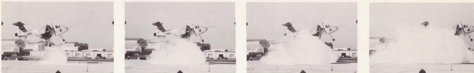
(b) 8 knots; 1.8 propeller diameters above ground; maximum power; out of ground effect.
