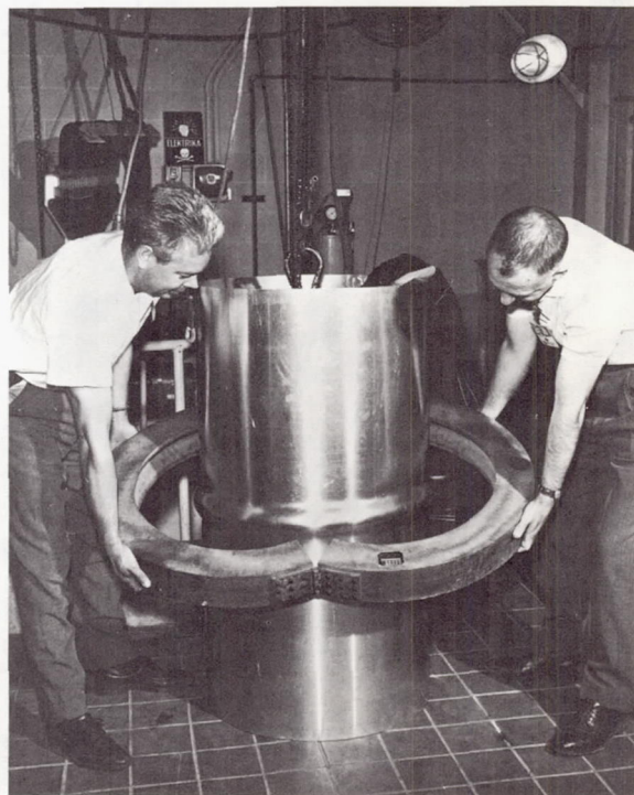
FIGURE 20-6.—Magnetic fields used to shape rocket tanks.
