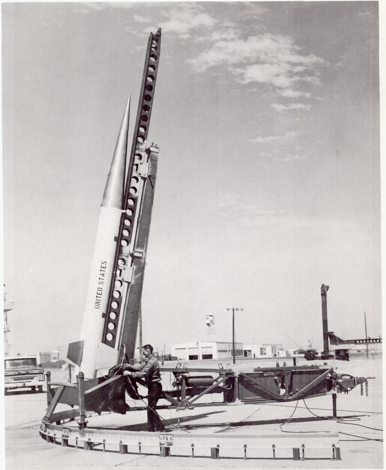
Figure 12.- Nike 10° cone on modified Nike-Ajax military launcher.
