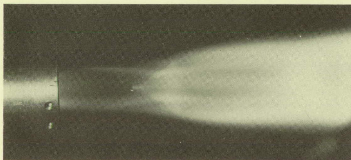
Figure 3 Overexpansion of Rocket Motor Flame Without Jet Separation
