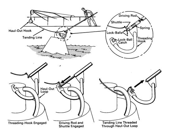
The problem: Attaching, with a minimum of delay and without hazard to an operating crew, a heavy-duty haul-out hook and cable used for emergency recovery of massive loads afloat in turbulent seas. The solution of this problem was particularly directed to the recovery from the sea of the manned five-ton Apollo command module when it returns to the earth after the Apollo spacecraft completes its lunar mission.
