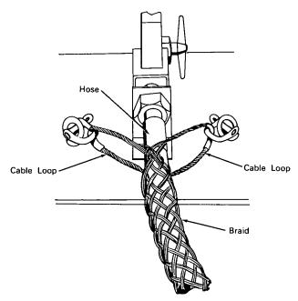
The problem: Failure amounting to rupture in fluid transfer hoses under high pressure can cause whipping action damaging to equipment and dangerous to personnel.
