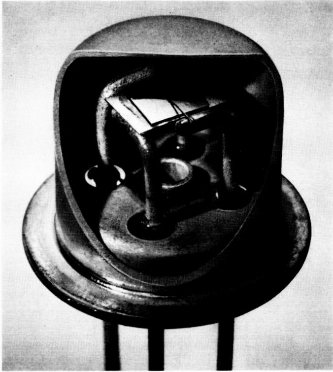
Fig. 6 — Construction of the radiation damage transistors.
