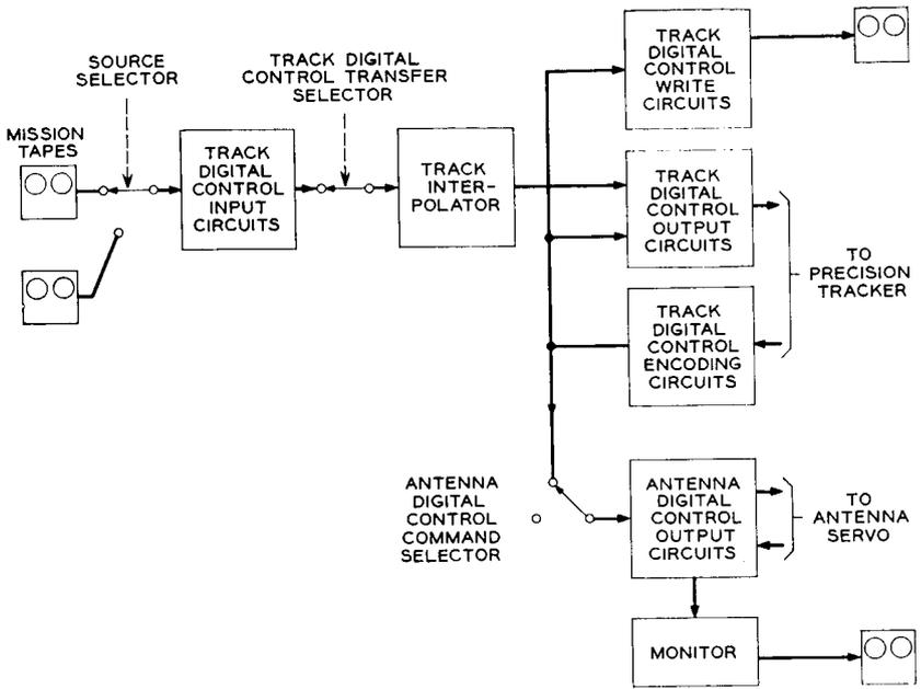
Fig. 9 — PT command mode operation block diagram.
