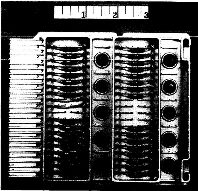
Fig. 11 — Logic package containing eight TRL gates.
