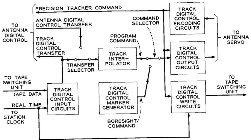
Fig. 7 — Track digital control block diagram.
