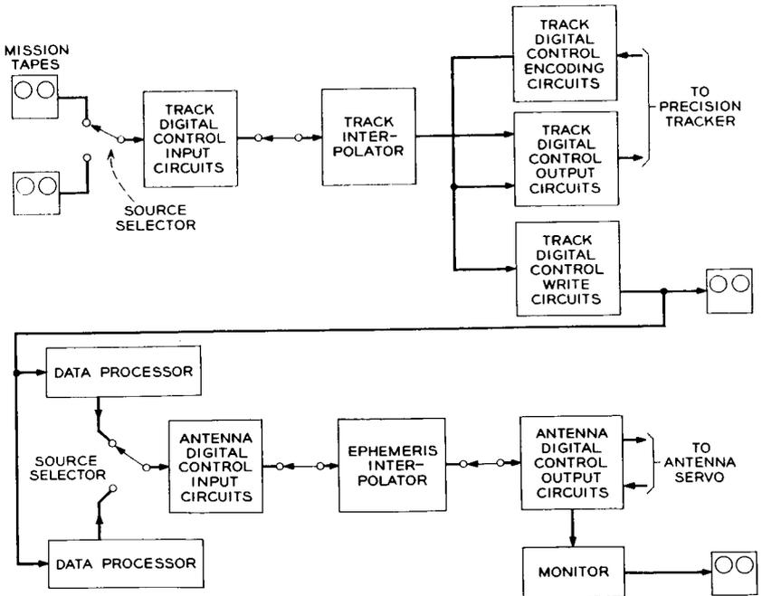
Fig. 10 — Initial mode operation block diagram.
