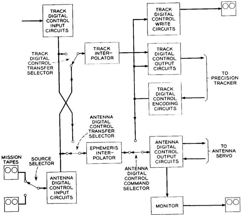
Fig. 8 — Normal mode operation block diagram.
