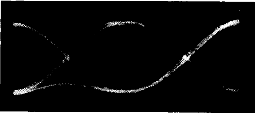
Fig. 47 — Eye pattern; 301A-XI Wideband Data Set. Satellite loop, pass 270, Aug. 8, 1962.
