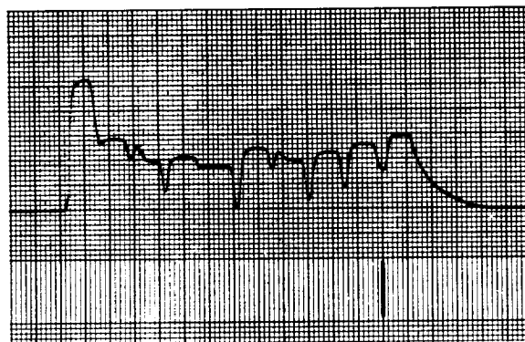
FIGURE 20-11.—Typical flight record showing operation of 10-channel solid-state switch.
