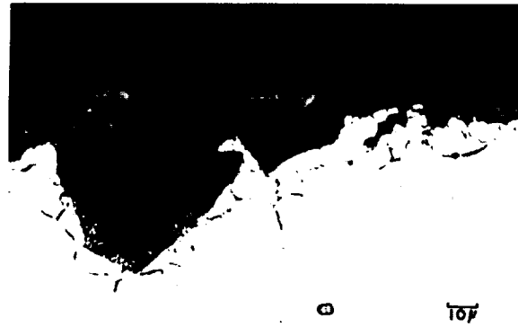
FIGURE 33-8.—Cross-sectional photomicrograph of oxide coating on Inconel X.
