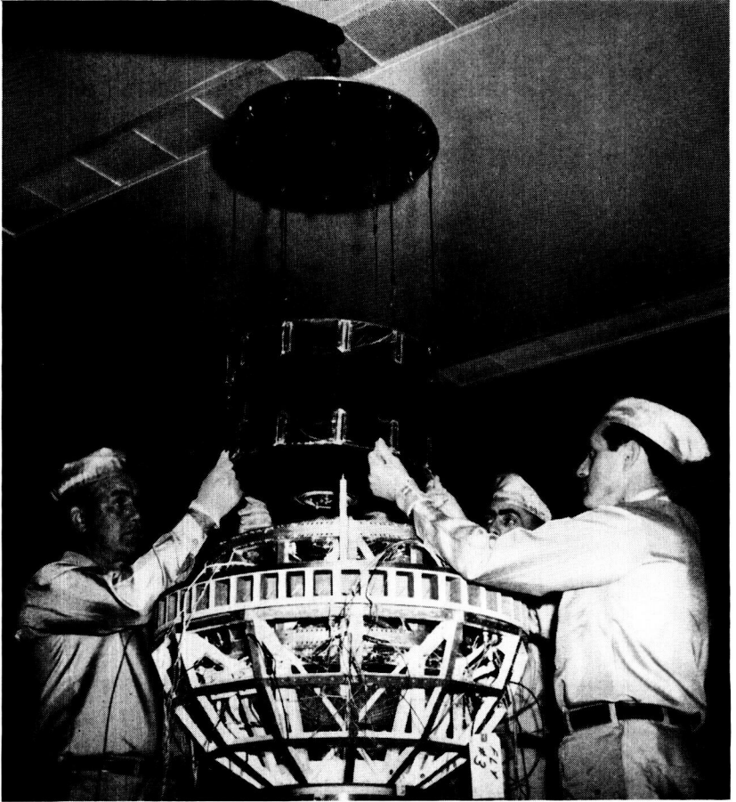
Fig. 9 — Mounting of electronics canister into the frame.
