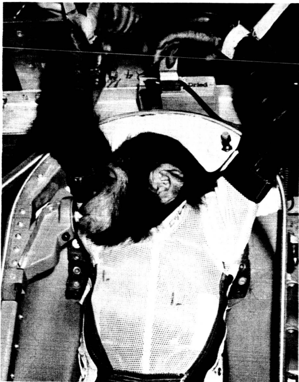
FIGURE 9-2.—An early training assembly showing the animal turning its head to obtain a drink. The green signal light appears just above the nipple.
