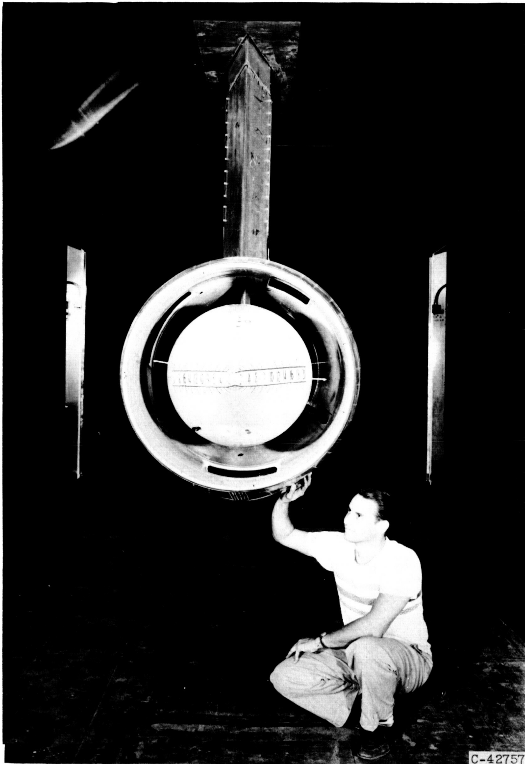
Figure 4. - Main inlet showing circumferential location of subinlets.
