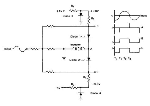
The problem: Clipper circuits are used in a wide variety of applications. Often, clipping action must start as the input voltage crosses the waveform zero axis (positive-to-negative or negative-to-positive transition point). Conventional transistor and diode circuits have been designed for this function but generally fail to maintain the start of clipping at the zero point.
