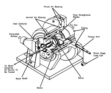
The problem: To absorb and measure power outputs (up to about 20 hp) of rotating machinery over an extremely wide range of shaft speeds—from 0 to beyond 75,000 rpm. Conventional air brakes, which consist of fans or air screws coupled to the output shaft, have the disadvantage of absorbing power in proportion to rotational speed. At low shaft speeds, very little power can be absorbed. At high rotational speeds, conventional air screws cannot measure low torques.
