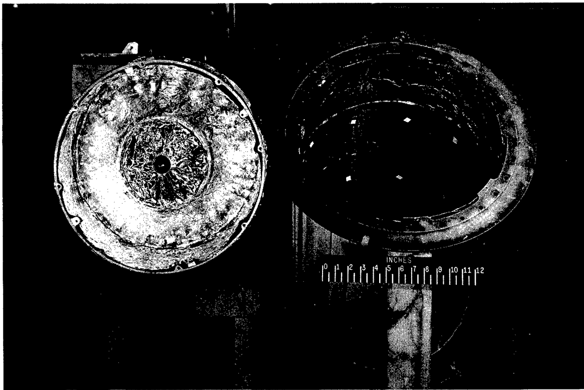
Figure VII-4.- Rocket-motor heat-transfer test; pressurized-cell mounting structure with aluminum foil on inside surface on the right and dome (forward end) of the X-248 rocket motor covered with aluminum foil.
