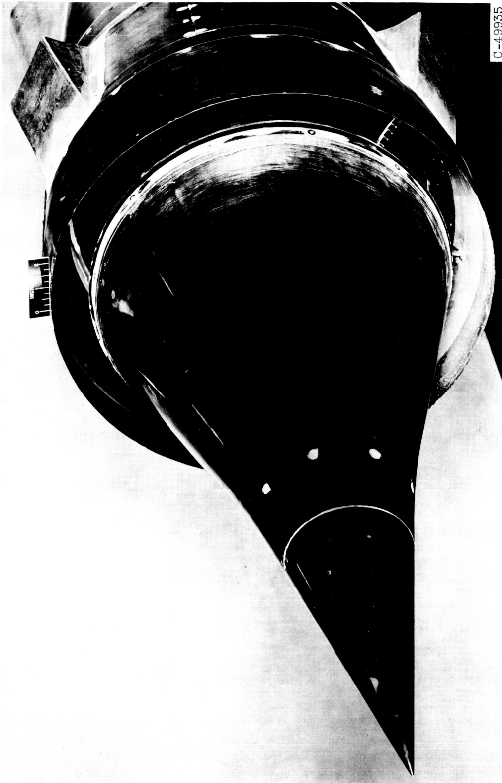
Figure 1. - Photograph of 19-inch isentropic two-step inlet.
