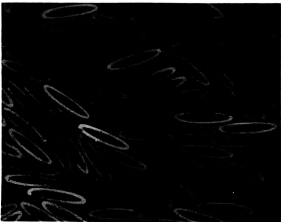
HOLLOW ELLIPTICAL FIBERS 5:1
