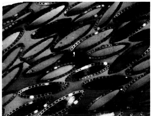
HOLLOW ELLIPSES WITH HOLLOW WALLS
