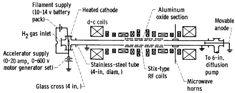
Figure 1. - Schematic of plasma source and ion-cyclotron resonance heating apparatus.
