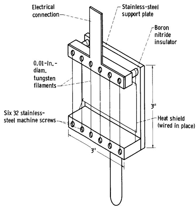
Figure 2. - Diagram of heated cathode.
