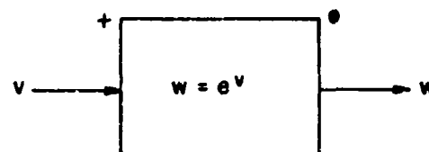
Fig. 2. Example of a homomorphic system with addition as the input operation and multiplication as the output operation.
