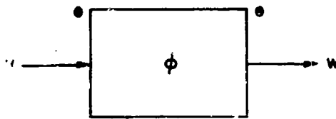
Fig. 3. Homomorphic system with multiplication as the input operation and output operation.
