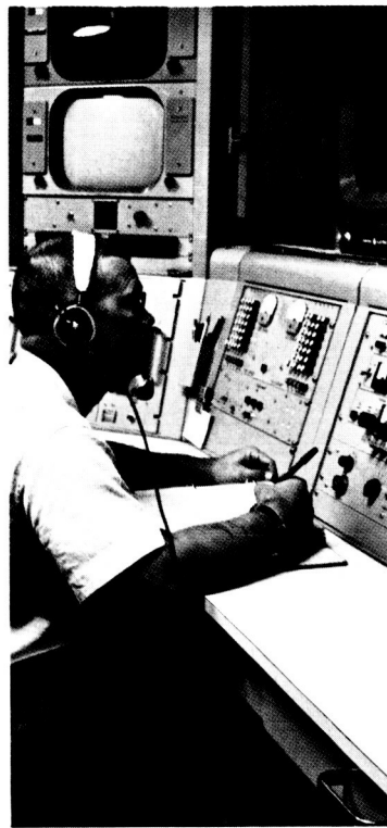
Signal is amplified and processed through the receiving system, and information from the signal is translated and recorded on magnetic and punched paper tape.
