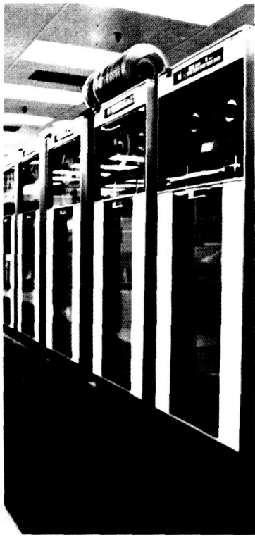
Processed data present video, tracking, engineering, and scientific telemetry in the form of time-labelled numerical printouts or graphs. All processed data are stored on magnetic tape.
