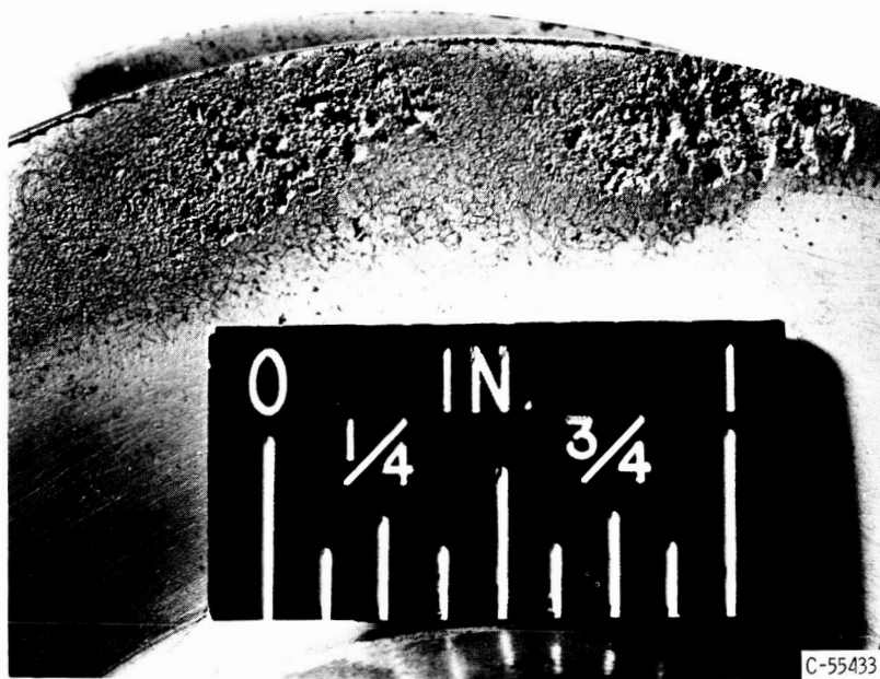
(b) Closeup of blade surface pitting.
